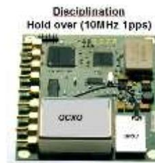
Providing GNSS time with a 1.5  $\mu$ s accuracy was “technologically simple” with such GNSS-LO devices, but holdover longer than a couple of days ask for ultraprecise oscillators ( high end OCXO, Rb oscillators), getting cost out of range...
